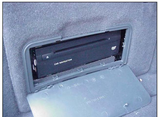
Figure 5 Insert DVD into Car Navigation Disk Drive
