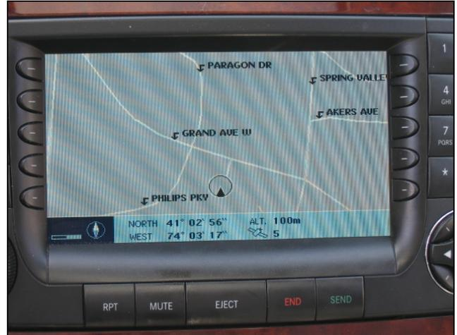
Figure 1 COMAND Display after pressing MAP key
