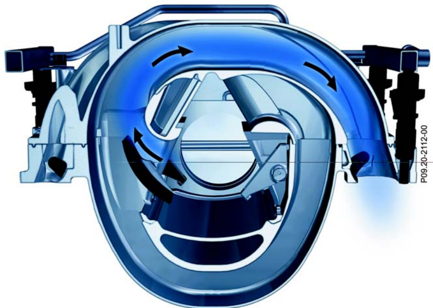
Routing flaps open, short intake channels
