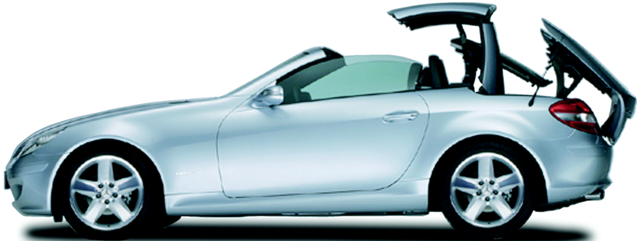
SLK retractable roof movement sequence (shown with accessory wheels)
