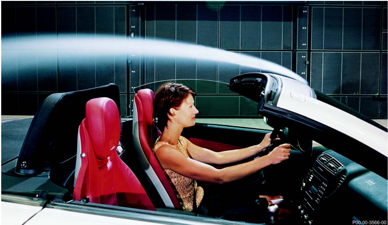
Airflow with retractable roof open
