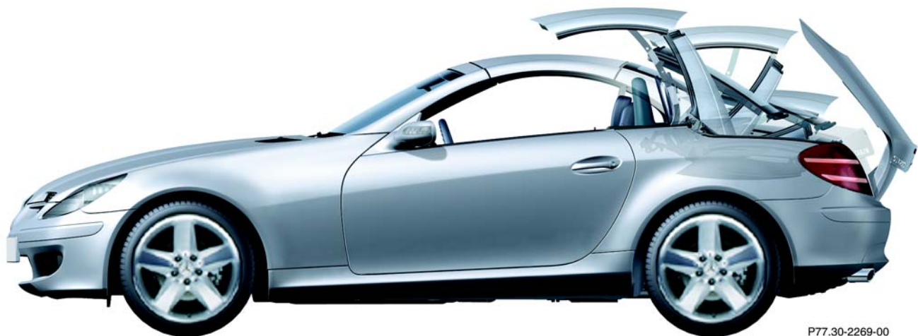
Retractable roof movement sequence (shown with accessory wheels)
