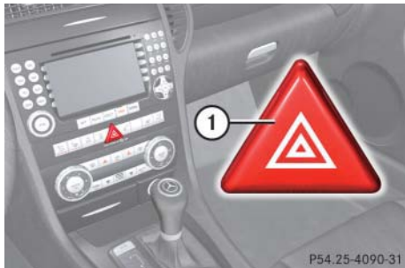
① Hazard warning flasher switch
