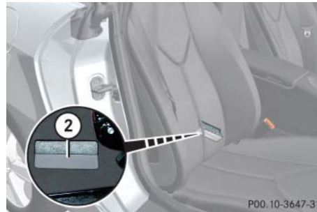
② Vehicle Identification Number (VIN), located behind the passenger seat under the floor cover
